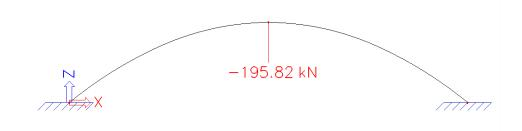
The buckling load N<sub>cr</sub> can then be calculated as:
