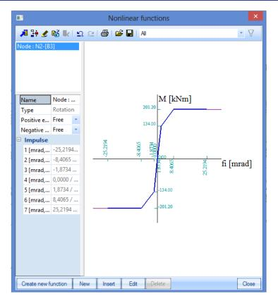
The function characterizes both tension-on-top and tension-at-bottom.
