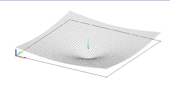
As can be seen, the slab will rise at the corners so no more tensile contact stresses are obtained:
