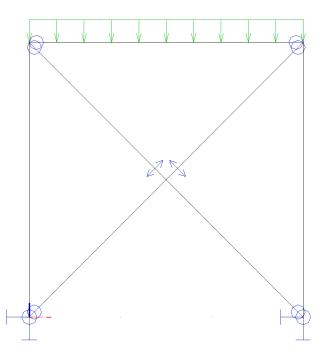
Due to for example a roof load, both diagonals are subjected to compression. This is not possible for **Tension only** members so both members are eliminated causing a global instability of the frame.
