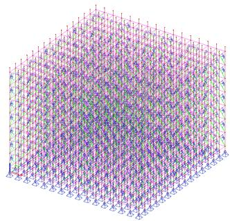
All diagonals of the structure have been given a gap of 1mm.
