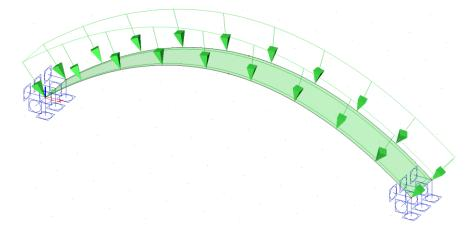
Using an Average Mesh size of 2D element of 0,1m, a Stability Calculation yields the following critical load factor:
