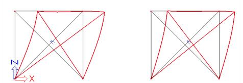
Due to the fact one diagonal has buckled in the left frame, larger horizontal deformations occur.
