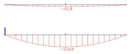
The following results are obtained for the normal forces in the cables:
