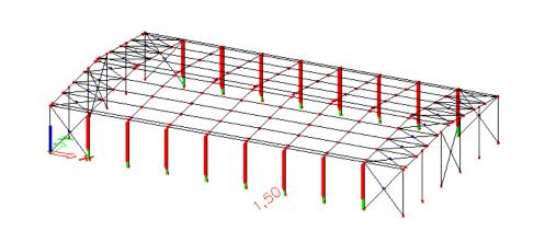
Since both global and local imperfections have been inputted, only the Section check and the Lateral Torsional Buckling check are relevant. In this example, member **B22** produces the largest check on the compression and bending check.
