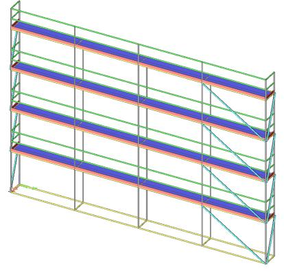
The base jacks are inputted as friction supports. Since a base jack, by default, is not connected to the surface, the Z-direction is defined as rigid **Pressure-only**. Both horizontal degrees of freedom X and Y are defined as **Friction**, dependent on the reaction Z.
