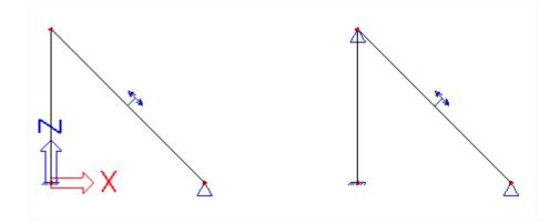
In the left frame, the Initial Stress will immediately be distributed to the column. In the right frame, the extra support will prohibit this.
