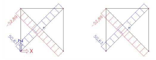
A **non-linear analysis**, taking into account the limit force gives the following results for the normal forces:
