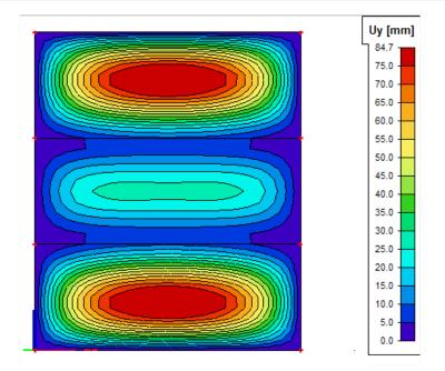
A **2<sup>nd</sup> Order** calculation using **Newton-Raphson** will take into account the development of membrane forces in the plate. These tensile membrane forces will have a positive effect on the stiffness on the plate and will thus reduce the deformations.
