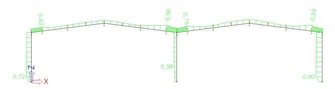
When **Path 2a** is followed, using a Global imperfection and a **2<sup>nd</sup> Order** Calculation according to **Timoshenko**, the Steel Code Check shows the following:
