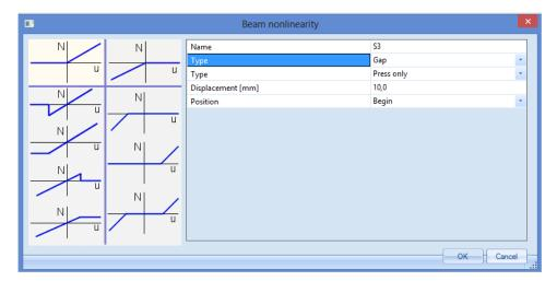
The **Type** field is used to specify if the member is active only in compression, only in tension or in both directions.
