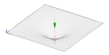
Especially in the corners, tensile contact stresses are expected:
