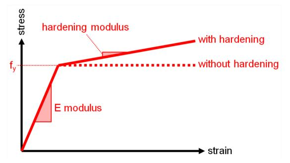
Only the tension part of the diagram is defined, as it is related to a plastification condition in general 3D stress state in principal stress directions. Some plastification models allow for a different yield stress in compression, which is defined separately. There is no limit (ultimate) strain value for the analysis.
