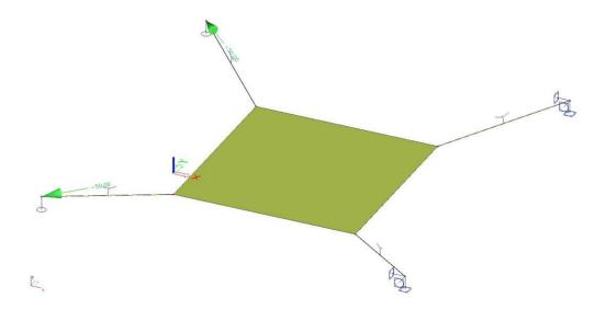
Since the canvas has an initial position **0,5m** lower than the endpoint of the cables, the canvas will first be pulled straight.
