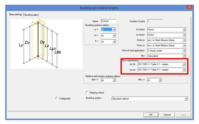
Since Global and Local imperfections are used for the columns, a buckling check needs not to be executed conform **Path 2c** of the diagram seen during the 2<sup>nd</sup> Order calculations. To take this into account in SCIA Engineer, the buckling factors can be manually set to a low value so buckling will not be normative.
