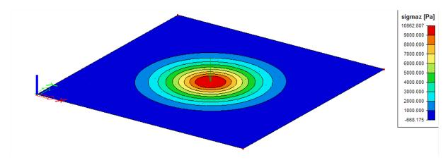
A **non-linear analysis**, taking into account the pressure-only characteristic of the subsoil shows the following deformation:
