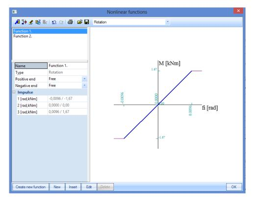
The beam-to-column connections are defined by the following non-linear characteristic:
