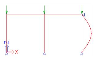
Buckling mode 2 – Critical load factor  $\lambda = 2,89$
