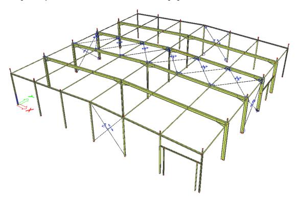
The structure is calculated in 2<sup>nd</sup> Order using **Timoshenko's** Method. The diagonals have been set as **Tension-only**.
