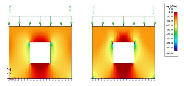
In these results the real pressure of this element is visible for the right element. Looking at the trajectories of this normal force, the trajectory of the pressure force will be even more visible:
