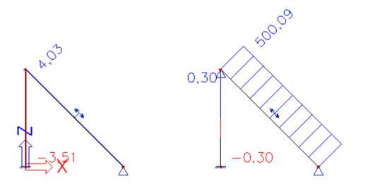
As specified, in the left frame, the initial stress is immediately distributed to the rest of the structure so the tensile force of 500 kN is not found entirely in the diagonal. In the right frame, the force cannot be distributed due to the support so the 500 kN stays in the diagonal.
