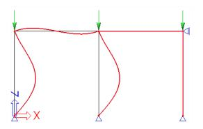
The loading F on each column is 100 kN so the critical buckling load  $N_{\mbox{cr}}$  can be calculated as:
