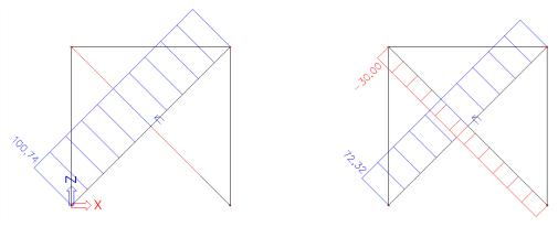
In the left frame, the diagonal has buckled so the tensile force in the remaining diagonal is augmented. In the right frame, the diagonal stays in the structure but yields plastically and thus acts at the limit force of -30 kN.
