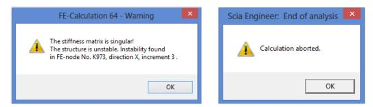
The singularity can be checked by running the check of singularities:
