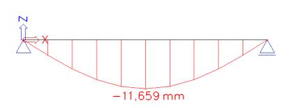
Due to the fact that the self weight causes this deformation, the compression force of 20 kN will lead to an additional moment.
