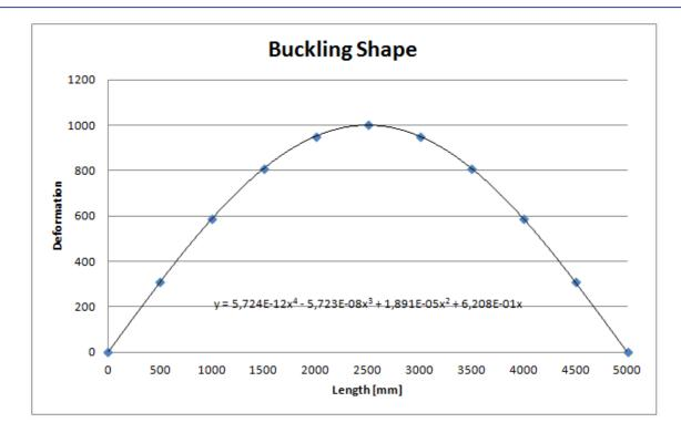
A polynomial has the advantage that the second derivative can easily be calculated.
