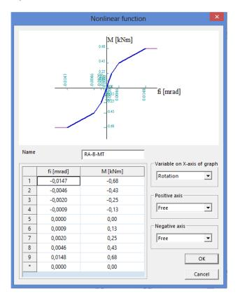
For member connections, the non-linear functions can be defined for translation or rotation. When defining a function, it is very important to check the signs of the function values. The defining magnitudes for non-linear rotation functions are the internal forces, for non-linear translation functions the displacements.
