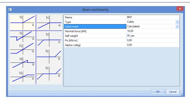
The initial shape will be in equilibrium in relation to the specified load on the cable: either the Self-weight or a distributed load **Pn**.
