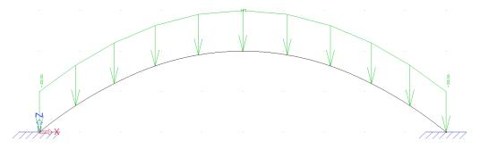
The Shear Force deformation is neglected to have a good comparison with analytical results. Using an **Average Mesh size for curved elements** of **0,1m**, a **Stability Calculation** yields a critical load factor of 0,46.
