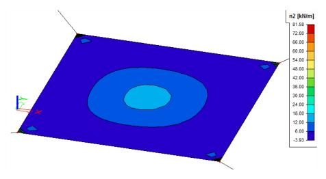
The results show the 2<sup>nd</sup> Order effect: due to the tensile forces in one direction, the canvas obtains a stiffness which results in compression membrane forces.
