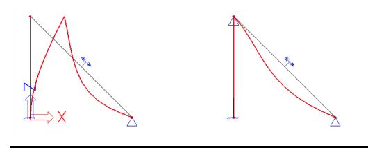
In theory, when using correctly defined values of the cross-section properties (surface A, moment of inertia I, modulus of Young E), a Beam non-linearity with Initial Stress can also be used to model straight cables with large pre-stress forces. Both **Timoshenko** and **Newton-Raphson** methods can be applied in this case.
