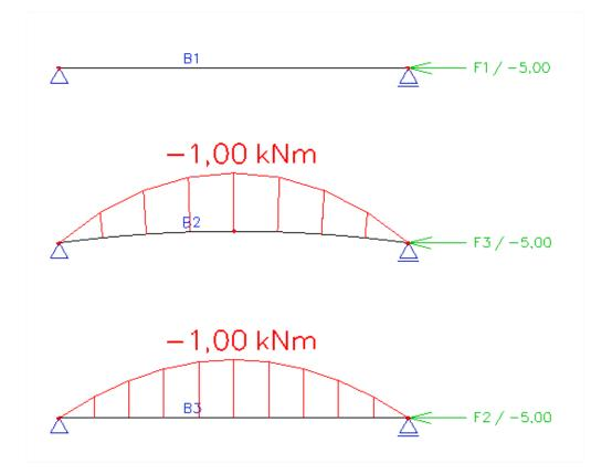
As expected, the beam B1 does not produce a bending moment. Both the curved beam and the beam with imperfection yield the 1 kNm.
