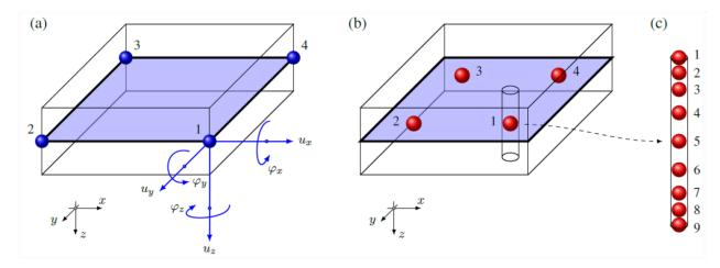
Due to these Gauss-Lobatto points the element can handle bending loading with high accuracy. In all of these points the nonlinear model is computed independently using the plane stress formulation. Linear transversal shear stiffness is assumed.
