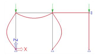
Buckling mode 3 – Critical load factor  $\lambda = 3,53$
