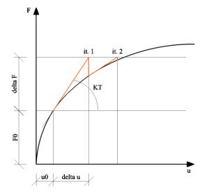
In this figure, the tangential stiffness  $K_T$  is used. The symbol u depicts the displacements and F is the force matrix.
