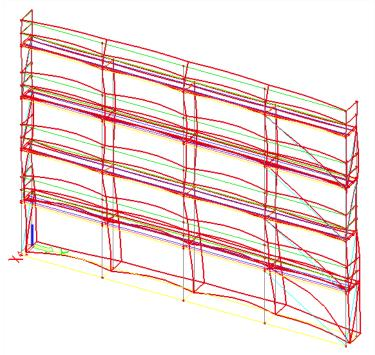
In the middle base jacks, the friction force is clearly surpassed and thus the supports slip through. To avoid this, the reaction in Z-direction must be augmented thus extra dead weight like ballast will be required or the base jacks must be fixed to avoid slipping.
